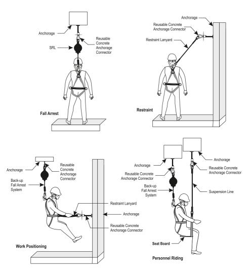
**INSTALLATION REQUIREMENTS:** For safe effective installation of the Reusable Concrete Anchor, make sure to observe the following requirements:
